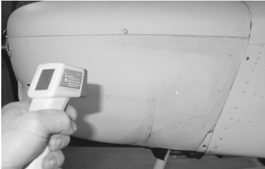
Left: the red laser dot is the centre of the sampled area. At this distance the sample is about 1.5" diameter
