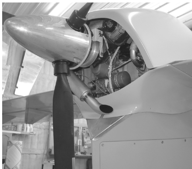
The Airmaster prop and engine fairing contribute to the speed range of the Nighthawk
