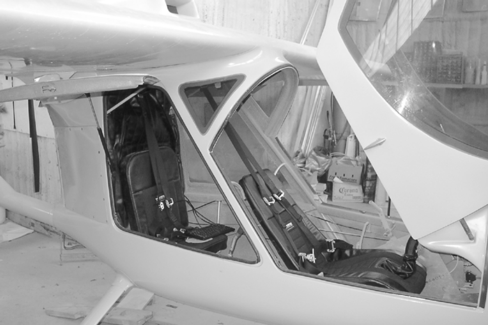
The larger rear seat is evident here. Electronics fit in the rear compartment. Note the aerodynamic shroud over the 912S
